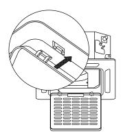
Connect the 2 wires of the decoration panel to the main board of the unit.
