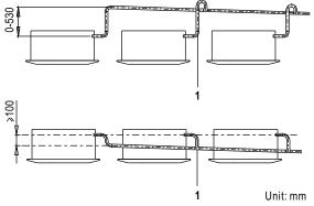
T-joint converging drain pipes
